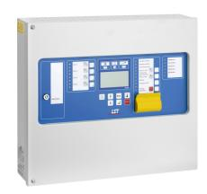
The compact Fire/Extinguishing Control Panel BC08 has been designed for use in single-zone extinguishing systems. Proven conventional technology allows the connection of automatic fire detectors, manual call points and contact detectors.
